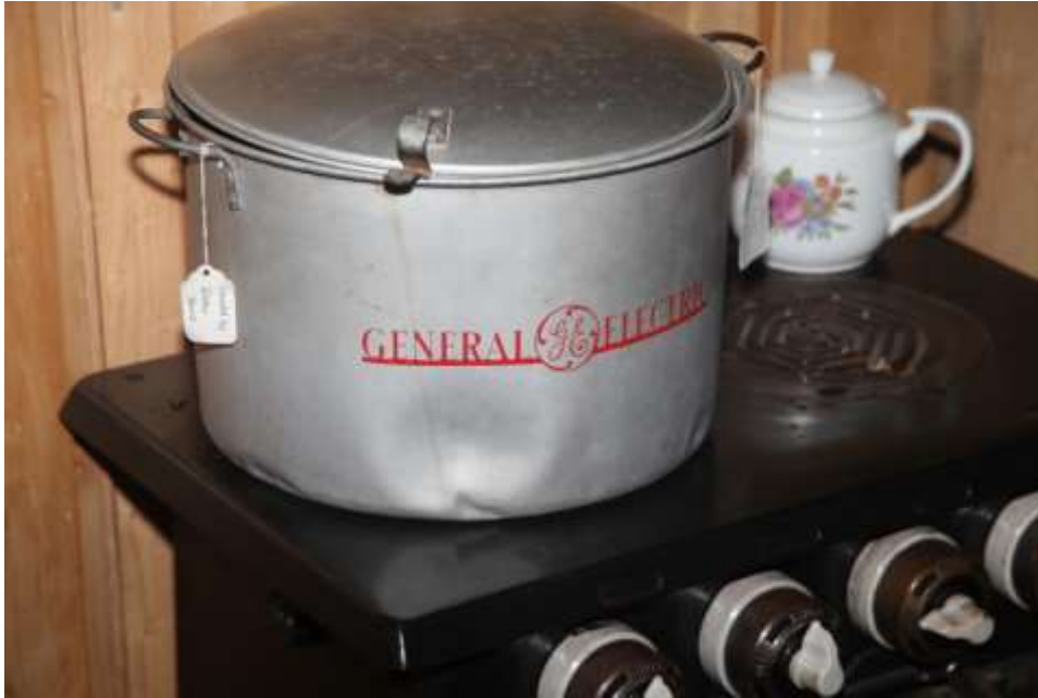
Part of a General Electric washing machine for sterilizing clothes of a tuberculosis patient. The bucket attached to an agitator on the washing machine.
