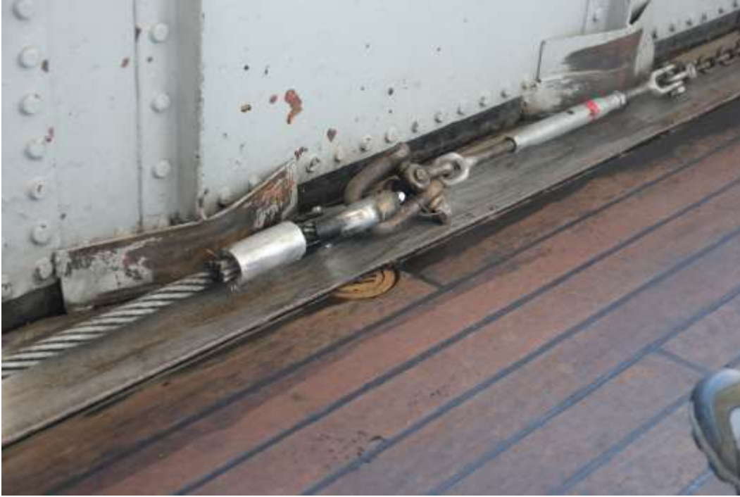
Exposed cable controlling steering
