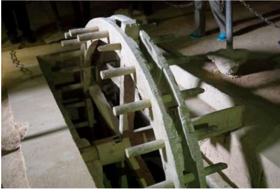
Mechanism to bring water up from underground stream
